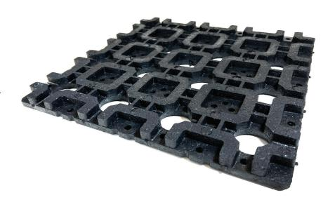
The Grid is designed to hold the pavers in place with the proper alignment and spacing. It enables quick and easy installation in up to a third of the time it takes to install traditional concrete or brick pavers. Grids are loose laid side-by-side, and the pavers interlock the system by overlapping adjacent grids.
